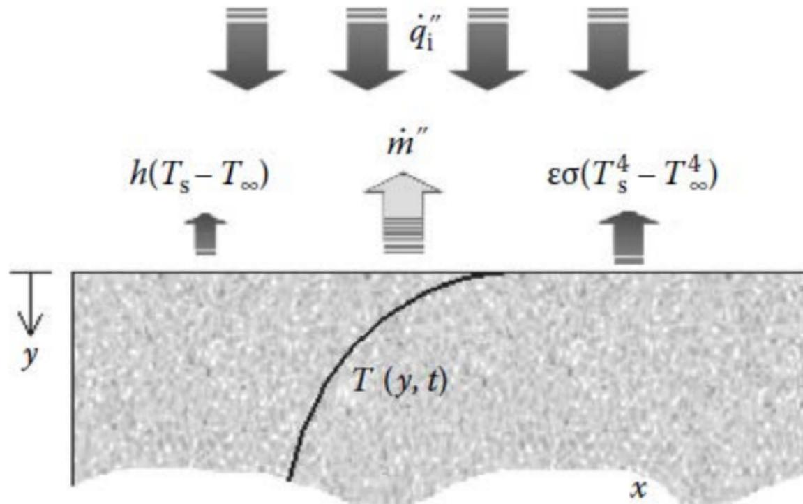
Figure 1. [Schematic of pyrolysis [12]]
