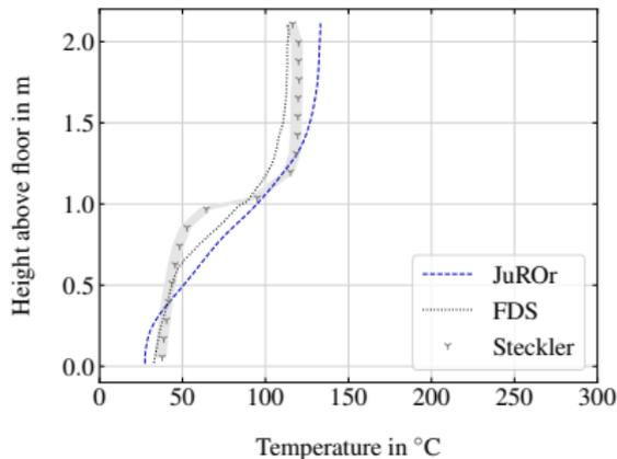
Temperature profile (at the bottom) at the center of the doorway
