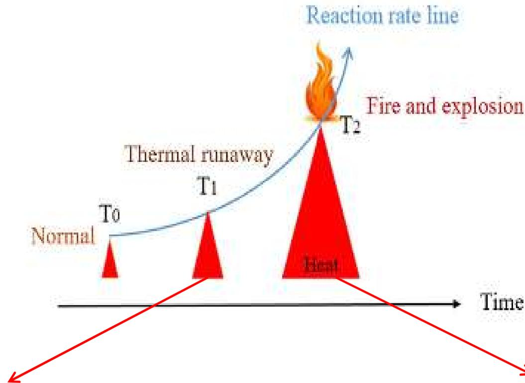
The risk of thermal runaway begins at a  $T$  of  $60^{\circ}\text{C}$  and becomes extremely critical at  $95\text{-}100^{\circ}\text{C}$ .
